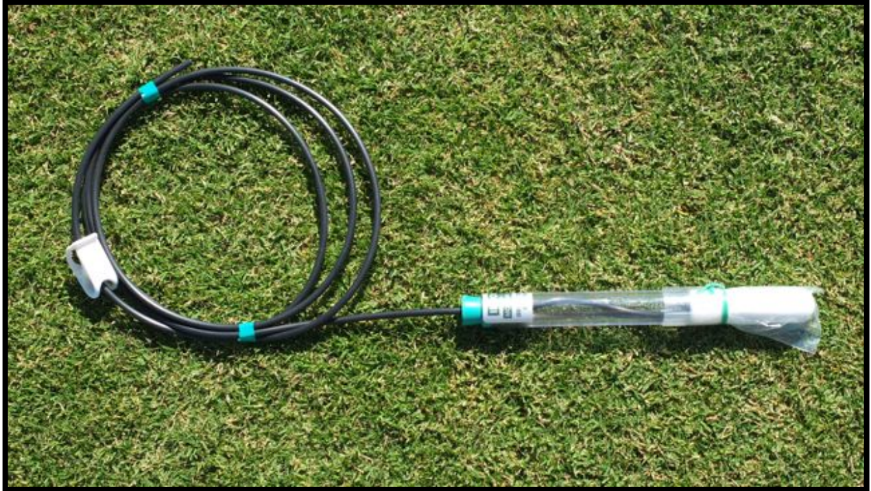
Figure 1. Suction lysimeters (Irrometer, Riverside, CA) used to capture leachate for analysis of EC_L . Lysimeters were buried 4 inches below the turf surface in 3 out of 6 replicate plots for each treatment.
